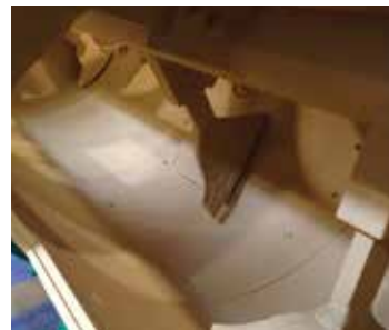
Chamber liner in special anti-wear material
