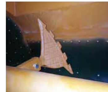
Special anti-wear mixing tool coating
